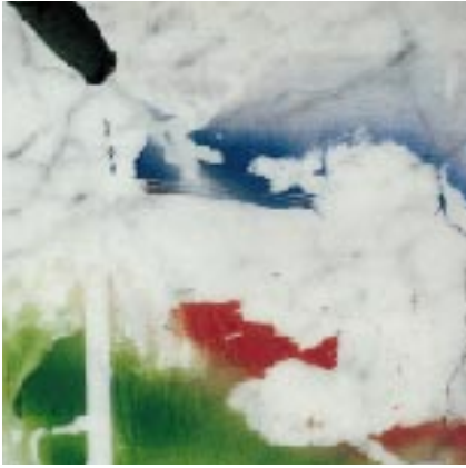
Using a high-pressure cleaner on Carrara marble treated with WallGard GRAFFITI BARRIER
