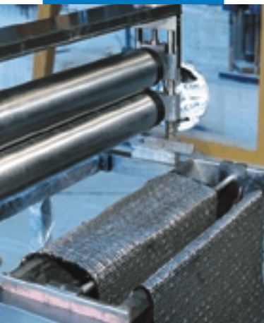
Mechanical impregnation of Mapewrap C
